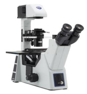
Inverted trinocular brightfield/phase contrast microscope, IOS
